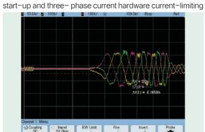
In the following figure, the hardware limits of the motor three-phase current is forced to flow through the inner limit point.
