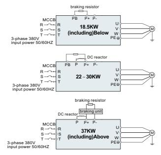
Figure 3-7 Main circuit wiring diagram
