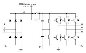
Figure 2-3 Main Circuit Diagram (over 30kw)
