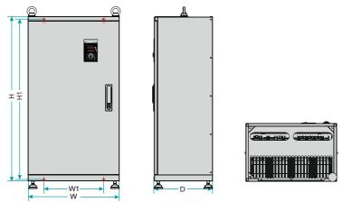
Figure 2-10 132KW~185KW AC drive installation dimensions and installation size
