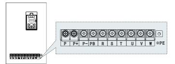
Figure 3-10 22kw main circuit terminal diagram
