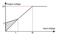
Torque boost to the output voltage for the features of low frequency torque. F04.01 is for the percentage of the rated motor voltage Vb. In practical application, torque boost should be selected according to the load. The bigger the load is, the bigger the boost is. Too bigger torque is inappropriate because the motor will run with over-magnetic, and the current of the AC drive will increase to raise the temperature of the AC drive and decrease the efficiency.
