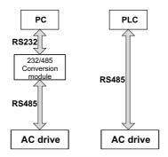
Figure 9-1 Single host/slave networking way
