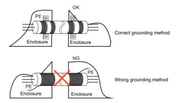
Figure 3-16 360-degree grounding technique diagram
