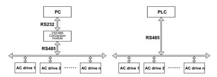
Figure 9-2 Single host/Multiple slaves networking way
