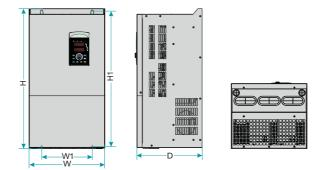
Fig 2-9 55~110KW AC drive installation dimensions and installation size
