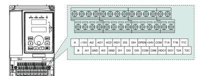
Figure 3-18 Control terminal diagram
