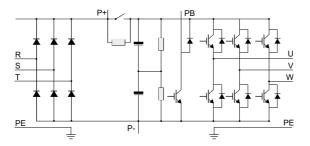
Figure 2-1 Main Circuit Diagram( less than 18.5 kw (including))
