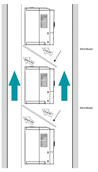
Figure 3-5 Vertical installation
