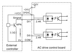
Figure 3-21 Sink wiring
