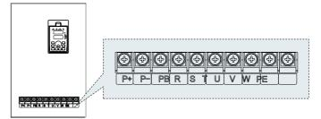
Figure 3-9 11~18.5kw main circuit terminal diagram
