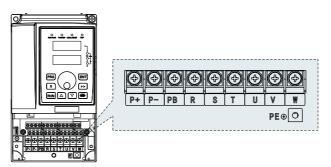
Figure 3-8 7.5KW below main circuit terminal diagram
