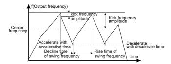
Swing amplitude is determined by F0A.00, when F0A.00, swing frequency is 0, means swing frequency is invalid.
