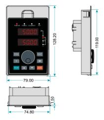
Figure 2-12 Keypad Installation dimensions
