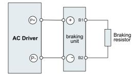
Figure 2-17 braking unit connection
