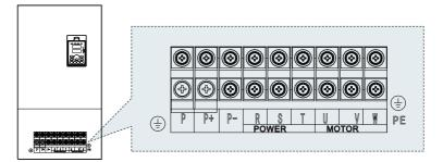
Figure 3-13 55~110kw main circuit terminal diagram
