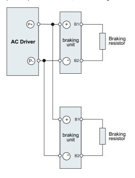
Figure 2-18 braking ones in parallel connection
