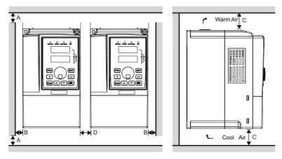
Figure 3-4 Parallel installation
