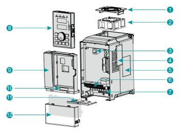
Figure 2-6 Product structure diagram
