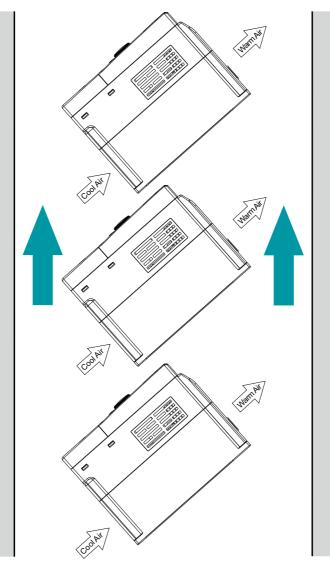
Figure 3-6 Tilt installation
