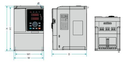
Figure 2-7 Less than 7.5 KW AC drive installation dimensions and installation size
