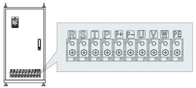
Figure 3-14 380V 132~185kw main circuit terminal diagram
