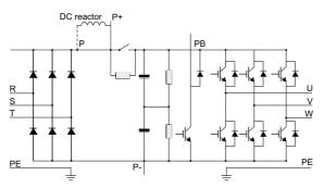
Figure 2-2 Main Circuit Diagram (22kw~30kw)
