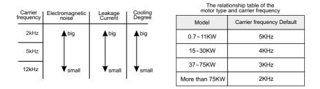
The advantages of high carrier frequency: ideal current waveform, little current harmonic wave and motor noise.
