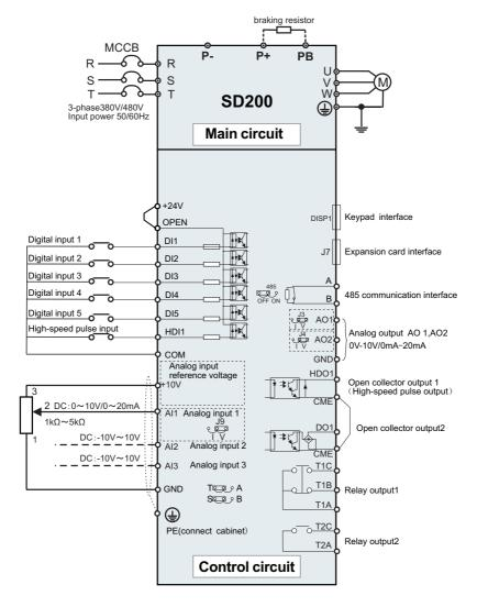
Figure 3-17 Wiring diagram of Control Circuit
