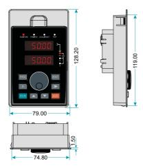
Figure 2-12 Keypad Installation dimensions
